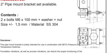
Foundation vibrations, as well as process vibrations, can disturb the proper functioning of the mounted instrument, the use of this bracket does not prevent or diminishes such occurrence.
